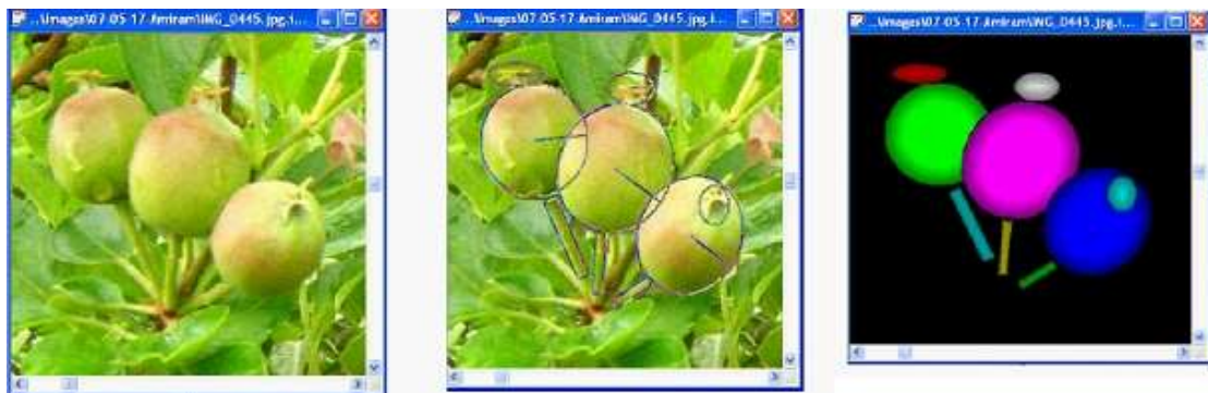
Figure 5: left: Original image. Middle: Image with objects marked by the user. Right: Image as seen by the algorithm (notice the objects relative depth and partial masking)
